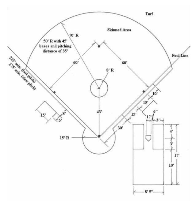
The measurements for a softball field(Above). The batter box measurements are the same for all age levels.
