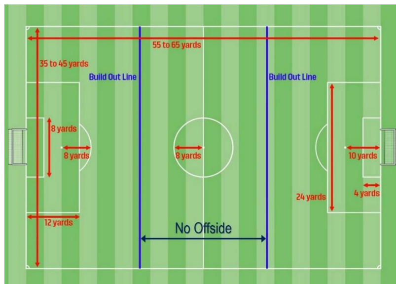
Figure 1. U.S. Soccer Field Standards and Markings for U10 Play Showing Build Out Lines
